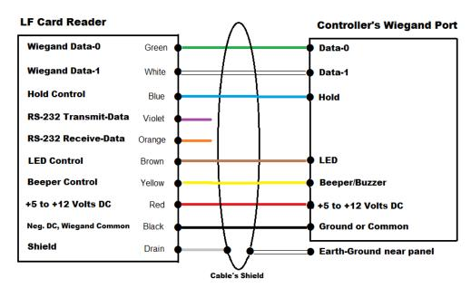
Note: The SR-2400 reader has no Hold control or RS-2232 interface. Do not use the **blue**, **violet** and **orange** wires.
