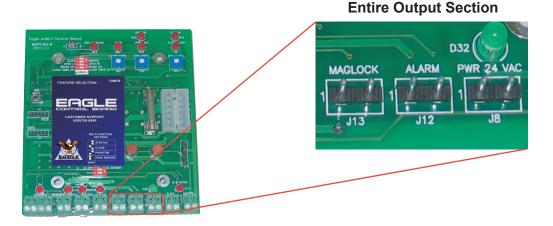
MAG Lock Solenoid Connections (24 VDC)
