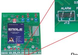
**Safety Alarm:** If the gate hits an obstruction twice while closing or opening, the system will shut down for 5 minutes. On the Board, you have two options of reset mode.
