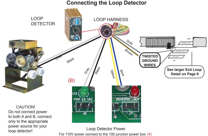
For 24V AC power connect to terminal on the Diamond Board (B)
