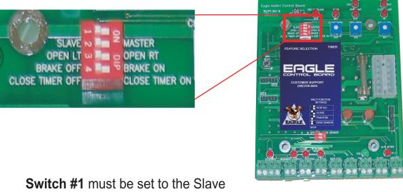
**Switch #1** must be set to the Slave or to the "off" position.
