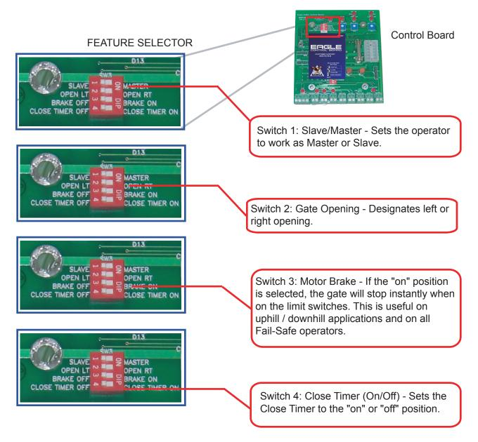
The reset button is used to reset the micropressor. IF YOU MAKE A CHANGE WITH THE SWITCHES, YOU MUST USE THE RESET BUTTON TO APPLY CHANGES. Note: If the power light is on and the operator does not function, press the reset button once. If this does not solve the problem, proceed with turning off the power switch and then switching it back on again.
