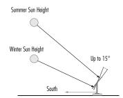
TIP: To optimize the system for winter operation the angle can be increased an additional 15° (solar panel(s) sits more vertical).
