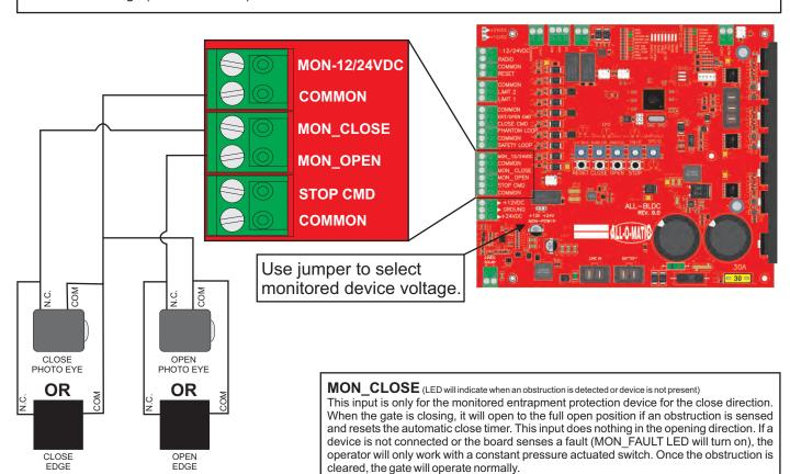
MON\_OPEN (LED will indicate when an obstruction is detected or device is not present)
