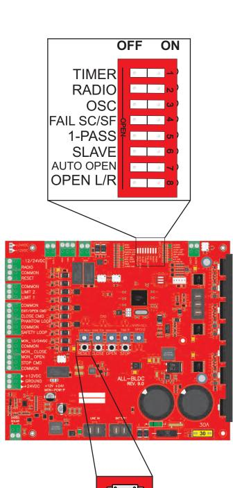
NOTE: IF ANY CHANGES ARE MADE TO THE DIPSWITCHES WITH THE POWER ON, PRESS THE MAIN RESET BUTTON TO RECOGNIZE THE CHANGES.
